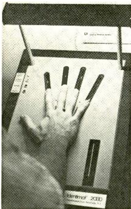
THE IDENTIMAT is a desk-mounted device that measures 13 x 19 x 19 inches, works unattended. It compares the information from the hand with that on the magnetic identity card, which is seen at lower right in the photograph.
